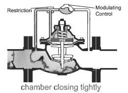
**Modulating valves** open and close based on pressure, like non-throttling valves. Modulating valves provide the following operations:
